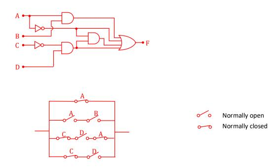
Figure 3: The  $F_2$  switching and logic schematics
