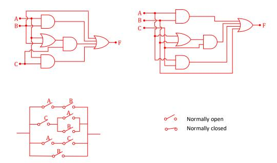
Figure 2: The  $F_1$  switching and logic schematics
